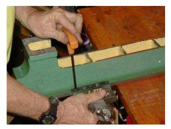
5. Snug up the six adjusting socket head cap screws to remove play, but allow the carriage to move freely.
