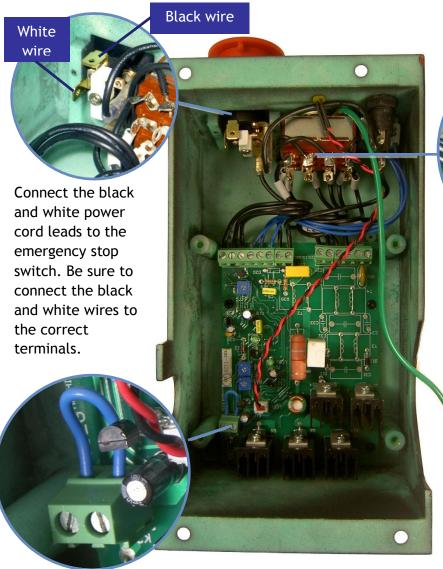
If your lathe has a safety switch (usually on a chuck guard) remove the jumper wire from the K3 and K4 terminals and connect the switch leads to these terminals. You can connect either lead to either terminal.
