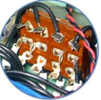
Connect the black and white motor leads to the F/O/R switch using the two terminals in the center of the switch. Connect either lead to either terminal. If the motor turns backwards from the way you have the switch set, simply swap the two wires.
