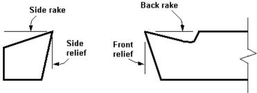
There is a cutting edge on the end of the tool bit called the front cutting edge. There is also a cutting edge on the side of the tool. Between these cutting edges is a rounded section of cutting edge called the nose.
