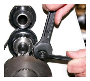
To change a gear in positions B or C, use an 8 mm end wrench on the square end of the shaft to keep it from turning. Loosen the nut with a 19 mm end wrench and remove the notched washer from behind the nut. Remove the nut so you can slide the gear off the shaft.
