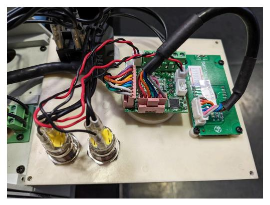
Solder two wires to each push button using the terminals shown on the drawing. The upper push button connects to the F/R terminals. The lower push button connects to the START terminals. The TAPPING terminals are not used.
