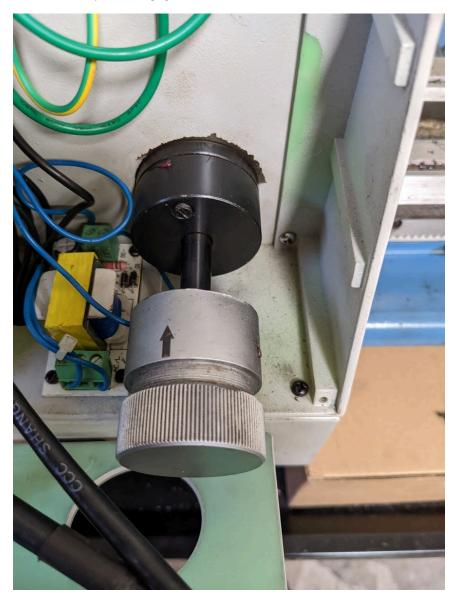
Install the spacer ring on the spindle to keep the gear engaged.
