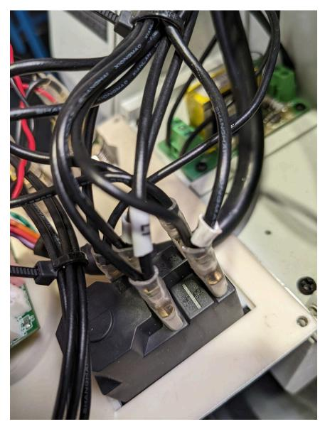
Replace the main control board and connect the new cable to it.
