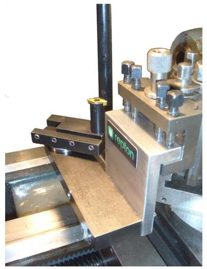
inboard. The zero radius point is where the radius slider is 27.2 mm from the inboard end of the rotating part. To turn a 10 mm radius, move the radius slider inboard until it is 17.2 mm from the end of the rotating part. Lock it in place with the locking set screws.
