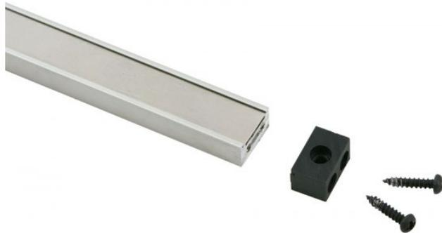
6. Install the two end caps. Note that there is a slot in the end cap that should align with the stainless steel strip. Use a Phillips screwdriver to secure the two screws in each cap.
