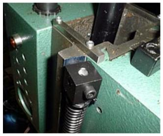
Drill and tap a 10-32 NF hole for the upper rack support block centered horizontally on the angled face from which you removed the scale. Position the block as high as you can on this face.
