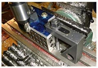
Move the step clamps as you work around the part. The two bolts will hold the bracket in position.
