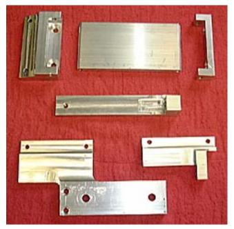
There are two alternates for mounting the X-axis scale. Use Bracket 3 if you do not have a mini mill power feed unit. Use Brackets 7 and 8 if you do have the mini mill power feed unit. Parts marked with a single asterisk (\*) are used without the power feed unit. Parts marked with a double asterisk (\*\*) are used with the power feed unit.
