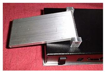
Mount the Display Arm on Bracket 4 using two 8-32 NC x 1/4 " self-locking dog point setscrews.
