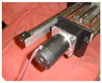
Sandwich bracket 8 between the mini mill power feed motor unit and the mill table. Use the existing socket head cap screws from the power feed unit to mount both the power feed and bracket 8.
