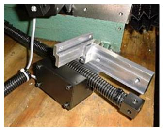
Using two  $\frac{1}{4}$ -20 x  $\frac{3}{4}$ " socket head cap screws, mount Bracket 1 on the left side of the carriage. The top of the bracket should be flush with the top of the
