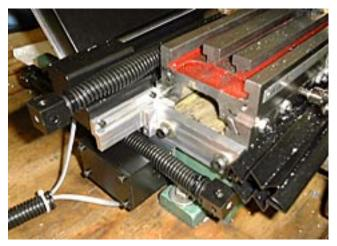
If you do not have a mini mill power feed unit, mount Bracket 3 on the end of the table, using an M6x16 socket head cap screw. Use the existing hole in the end of the table.
