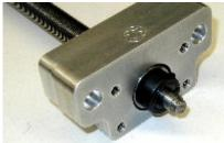
12. If any of the above conditions exist, loosen the setscrew and repeat the previous four steps until the lead screw rotates smoothly with no noticeable axial or radial play.
