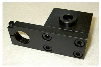
When you receive your rotary tool mount the spacer might be clamped in the hole for the Proxxon rotary tool.
