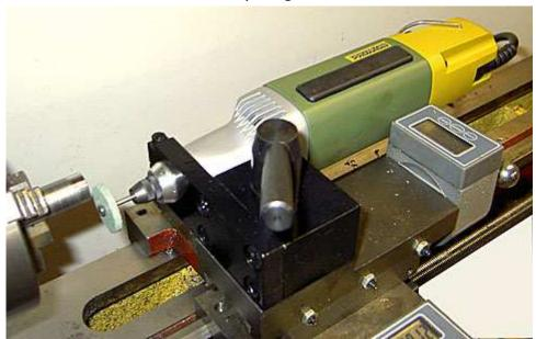
The Proxxon rotary tool mount replaces the tool post on your mini lathe. It includes a spacer so that the standard tool post stud and handle work to retain it.
