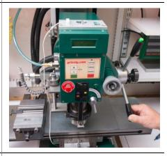
Gently tug on the Safety Switch wire to make sure that it is not pinched between the mill head and Control Panel.
