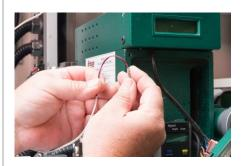
19. Disconnect one wire from one of the E-Switch lugs.
