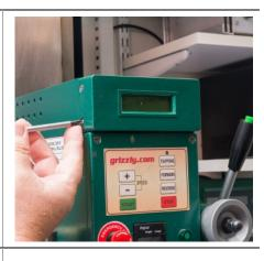
3. Unscrew and remove the Spindle Cover.
