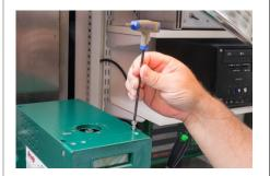
14. Unscrew and remove the Hub & Lock Bolt on the lower right corner of the Control Panel.
