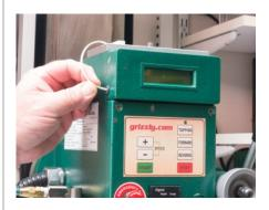
26. Test the operation of the Spindle Brake. Slide the Spindle Brake Disc down over the top of the drawbar and spindle. With the Spindle Brake Disc correctly in place, the spindle should be locked and the power to the mill cut. When lifting the Disc off of the plate, power should return to the mill.
