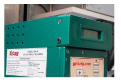
9. Remove the 2 front M5-.8 x 40MM cap screws from the Belt Cover on top of the mill.
