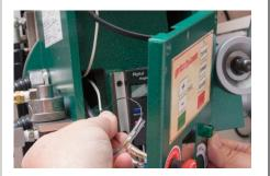
24. Reinstall the Hub & Lock Bolt on the lower right corner of the Control Panel.
