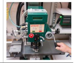
16. Remove 4 M4-.7 X 16MM flat head machine screws holding the Control Panel. Carefully remove the Control Panel and gently let it hangdown below the mill head.
