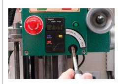
Make absolutely certain that the wires leading up into the notch on the top left of the Control Panel and the bottom left of the display housing are not pinched between the mill head and Control Panel.
