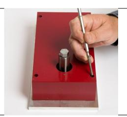
8. Install the safety switch to the Spindle Brake plate using the 2 supplied #4-40 x 1/4" pan head machine screws.
