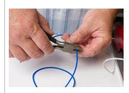
11. The safety switch will now be spliced into one of the wires connected to the Emergency Switch (E-Switch).
