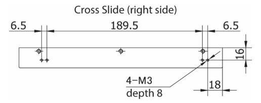
2. Drill and tap the four holes M3. Use a 2.5 mm or #39tap drill and an M3x0.5 metric tap.
