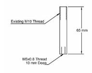
Use an M5 x 20 set screw to mount the stud to the cross slide.
