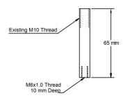
Use an  $M6 \times 20$  set screw to mount the stud to the compound rest or cross slide.
