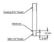
Use this stud to mount the OXA QCTP to the compound or cross slide. If there are two tool post mounting holes, choose one of them to mount the OXA QCTP.
