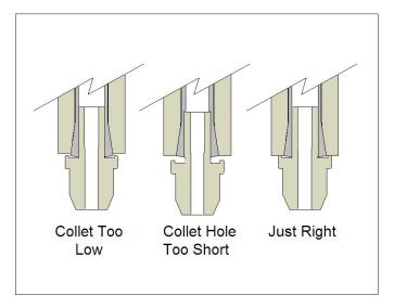
The center diagram shows a collet where the 3/4" section inside the collet is less than the length of the TTS shank. This will also prevent the shoulder from contacting the face of the spindle. If the shoulder cannot make contact with the spindle face, then the unique benefits of TTS (rigidity and exact Z height) will not be seen.
