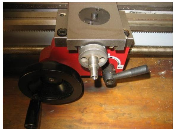
18. Replace the graduated dial and spring. Put the graduated dial onto the shaft leaving the spring groove exposed.
