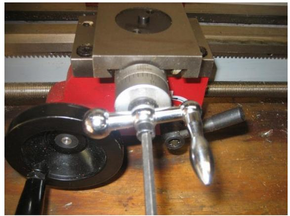
21. Replace the compound rest. There are two socket head cap screws.
