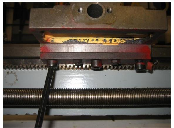
7. Reattach the apron to the saddle. There are two socket head cap screws.
