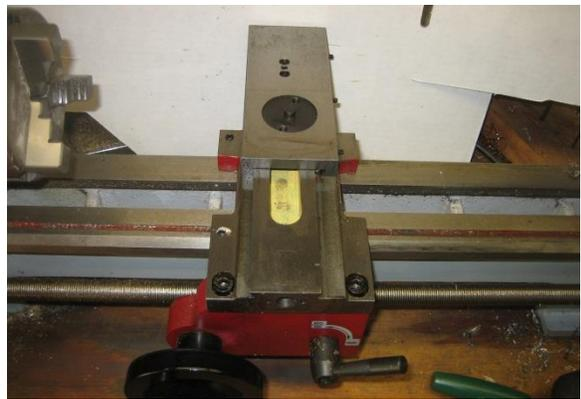
7. Detach the apron from the saddle. There are two socket head cap screws.
