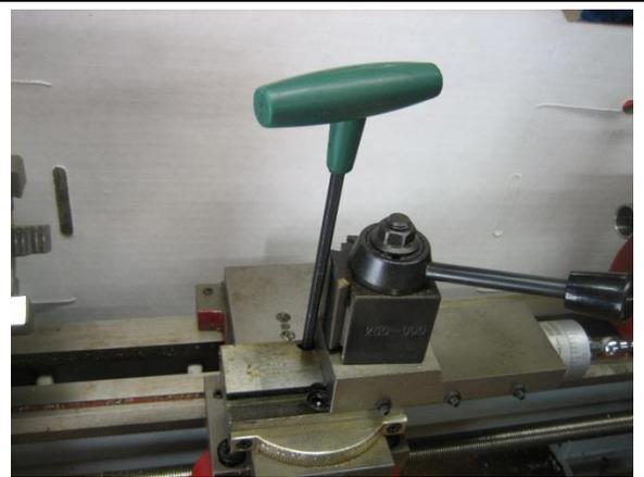
2. Remove the hand crank from the cross slide. There is one socket head cap screw. Note the position of the washers and spacers.
