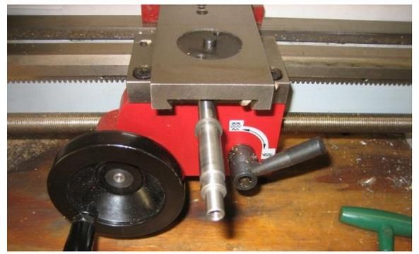
6. Loosen the gib adjusting screws and slide the cross slide off the saddle to remove it.
