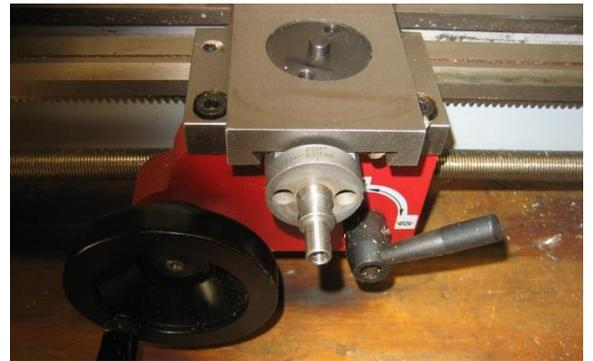
5. Unscrew the feed screw to remove it. It is a left hand thread.
