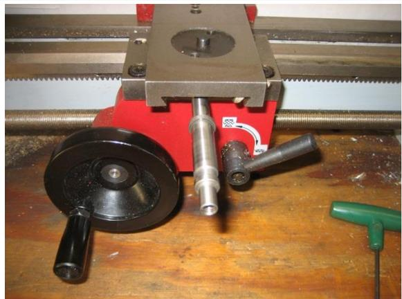
17. Replace the cross slide screw retainer. There are two socket head cap screws.
