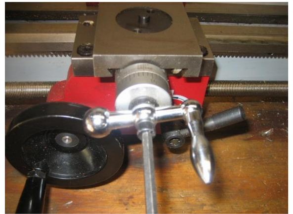
4. Remove the cross slide screw retainer. There are two socket head cap screws.
