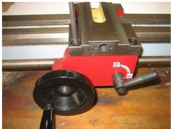
8. Remove the front and rear saddle retainers. There are six socket head cap screws.
