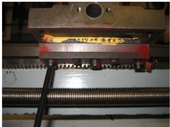
9. Remove the set screws from the follower rest mounting holes. Remove the saddle from the ways.
