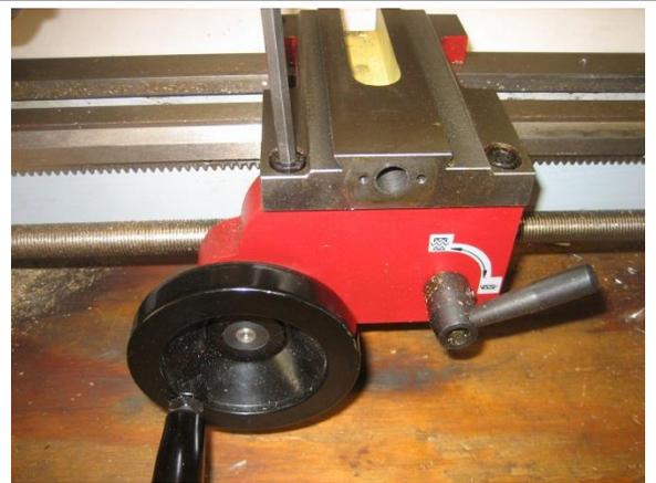
8. Loosen the three lock nuts on the side of the cross slide.
