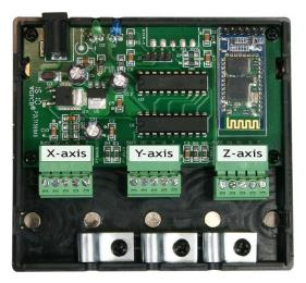
Install a green plug on the wire from each read head. With the screw heads up, the colors, from left to right are: Red White Yellow Brown Gray
