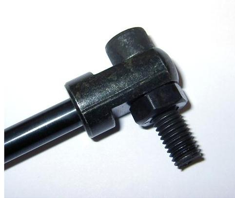
6. Put an M10 nut on each end of the head support shaft.
