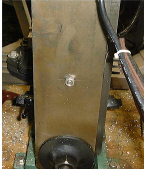
3. Drill and tap two M6 holes into the top of the spindle housing mount casting positioned as shown on the Air Spring Mounting Holes drawing at the end of this document. Use a 5.0 mm or #9 (0.196”) drill bit. Use an M6x1.0 tap to thread the holes.
