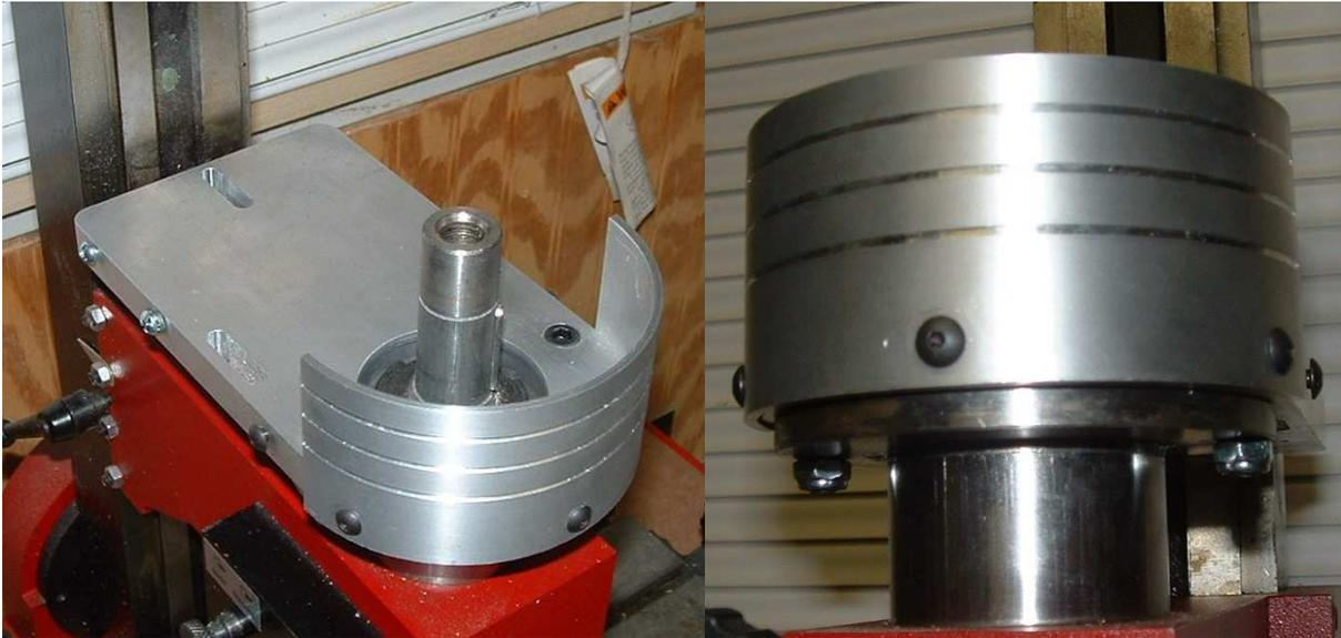
12. Insert the key in the key slot on the spindle, and slide the new spindle pulley onto the spindle, large pulley toward the plate.
