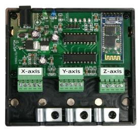
Install a green plug on the wire from each read head. With the screw heads up, the colors, from left to right are:
