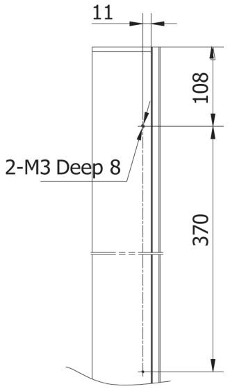
4. On the left side of the column housing, mark the two hole locations as shown below. These are clearance holes for the Z-axis scale mountings, so be sure they will align with the two holes in the column. Notice that these holes are large enough (10 mm) to provide clearance for slight misalignment.
