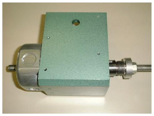
11. Tighten the nuts on the threaded rod to press the spindle (item 79) out of the spindle box (item 49) and top bearing. The spindle might come out together with the lower bearing. This is preferred.
