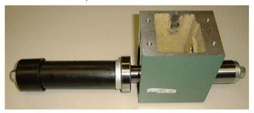
• If you don't have the R8 Spindle Installation Kit, place the bored 3/4" washer over the top of the spindle. Put the 5" long section of 1-1/2" pipe and cap over the top of the spindle, followed by one or two 1/2" flat washers and a 1/2" nut, as shown below. Don't forget the 3/4" washer. You will crush the bearing shield without it.
