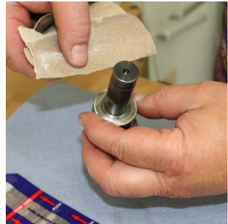
Figure 14. Lightly sand the tool in preparation for conversion
