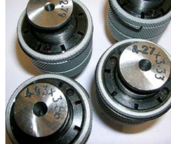
Figure 9. Collet sizes are displayed as Hole Diameter (mm) x Square Size (mm)
