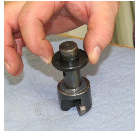
Figure 17. Place the conversion ring on the tool
