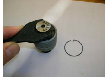
Figure 11. Once the spring clip has been removed, the spanner can be used to tighten or loosen the adjustable nut.
