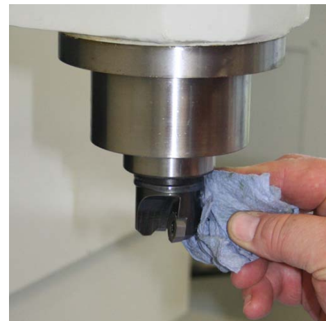
Figure 18. Clean the epoxy residue the tool
