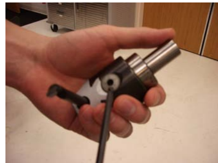
Figure 6. Adjusting the boring head
