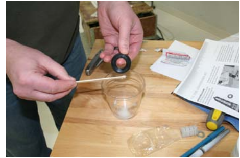
Figure 16. Spread the Epoxy on the conversion ring
