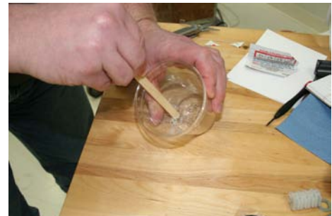
Figure 15. Mix the epoxy. Avoid skin contact
