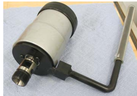
Figure 7. Reversing Tapping Head with Brake Rod installed.
