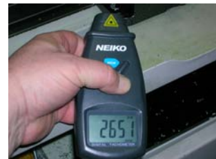
Figure 12. Use a Tachometer to accurately measure spindle RPMs. Mark the spindle with reflective tape and aim the tachometer at the mark with the spindle running to measure RPMs.
