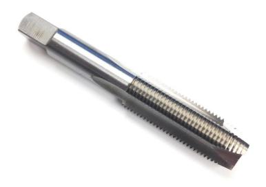
Spiral point taps are generally used for through holes. They have a very short spiral on the cutting face of the first few threads. This "shoots" the chips out the bottom of the hole, thus they are sometimes called "gun taps." Because spiral point taps do not have to be reversed, and because the shallower flute passages provide a greater cross section to the tap, they are favored for machine tapping of through holes with all materials.
