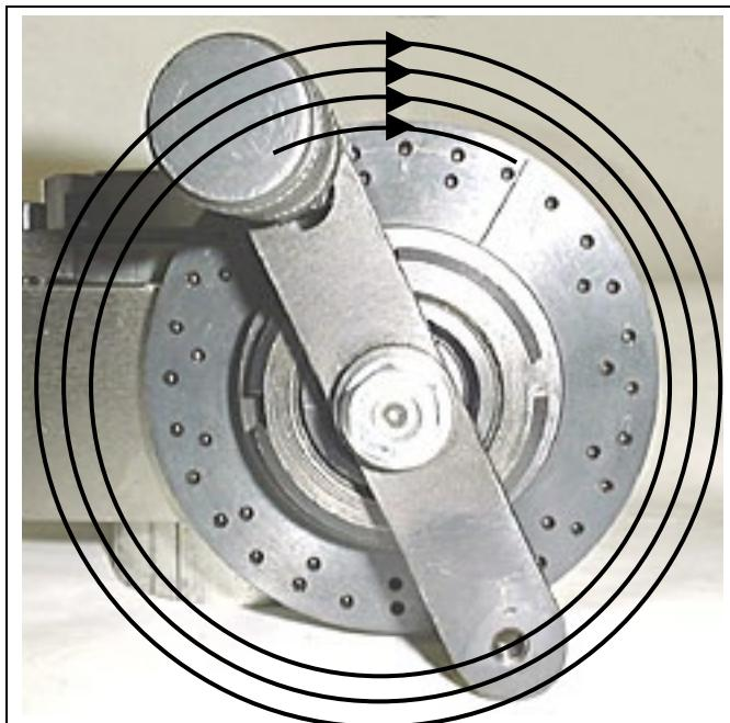
This shows rotating three complete turns, plus advancing 4 additional holes to the right sector arm.
