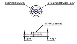
We can't tell you the dimensions, except that the center hole must be tapped M10x1.50 thread. The tap is our P/N 4838. Measure your T-slot and make it an easy fit.
