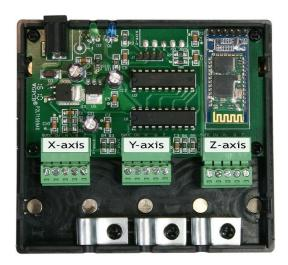
3. Install a green plug on the wire from each read head. With the screw heads up, the colors, from left to right are:
