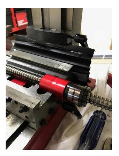
Use the long 6mm screws that came with the kit. Put the extension on and also the end cap from the handle end. Use the existing thrust bearings
