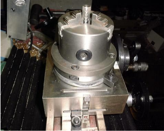
Lathe chuck mounted on a rotary table
