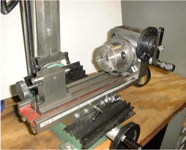
Rotary table set up for indexing with a tailstock
