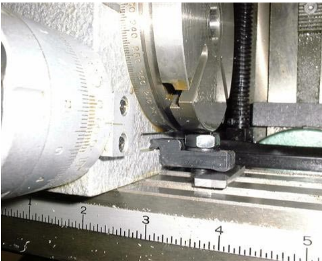
The rotary table mounted vertically.
