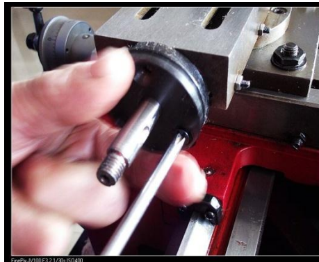
6. Mount the connecting plate from the DRCD Kit.
