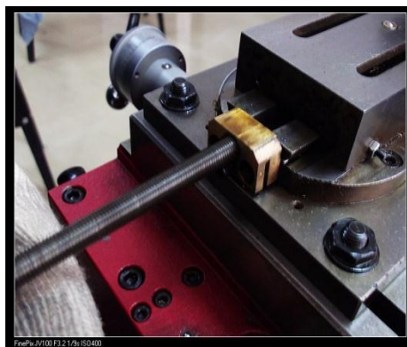
4. Install the leadscrew from the DRCD Kit.
