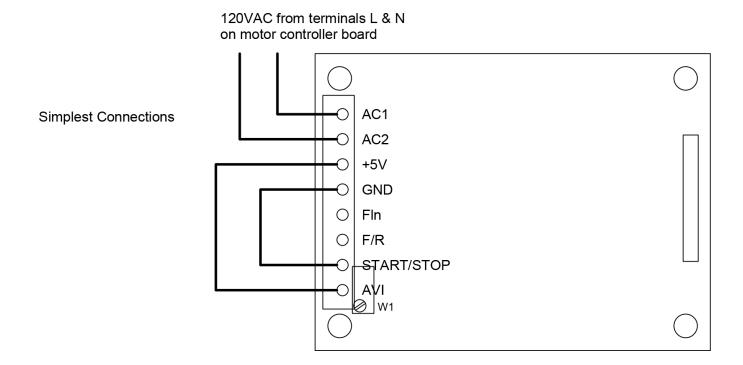
There are several wiring diagrams included in this document. After running the motor with the Simplest Connections, you can proceed to make connections to your breakout board.
