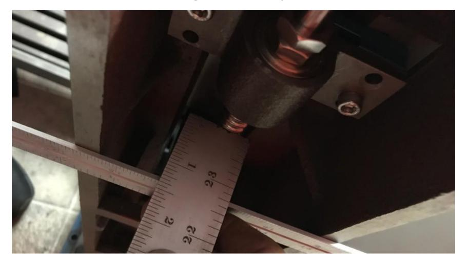
Now you can take a measurement from the back of the machine to the ball screw. Add ½ of the diameter of the ball screw to that measurement and transfer to the top of the casting. This is where you will drill the hole for the motor shaft.
