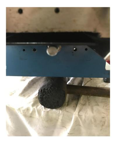
They will want to get hung up on the machined flat where the y block bolts down. Slide the saddle on just a little.
