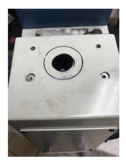
When you put the Z motor mount on, you can make any adjustments through the hole where the other handle was.
