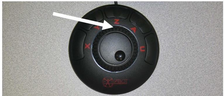
3. The inside dial has detents, or “clicks.” Each click to the right will jog up one “Cycle Jog Step” increment as configured in Mach3. Conversely, each click to the left will jog down one step. To see the step increment setting, hit the “TAB” key, and the graphic on the right will appear. To change the setting,
