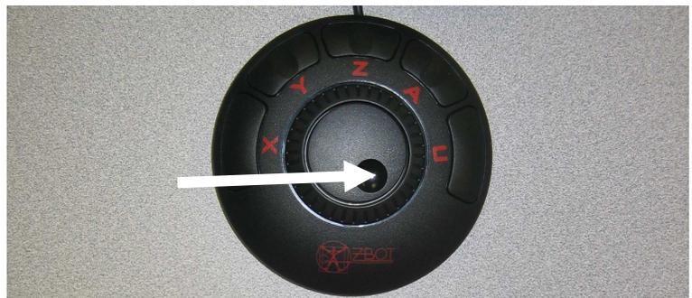
either hit the “Cycle Jog Step” button on the screen, or configure the “U” button on the jog dial to “Cycle Jog Step”. It is common practice to get close to the desired location with the outside dial, and then switch to the inside dial for final positioning.
