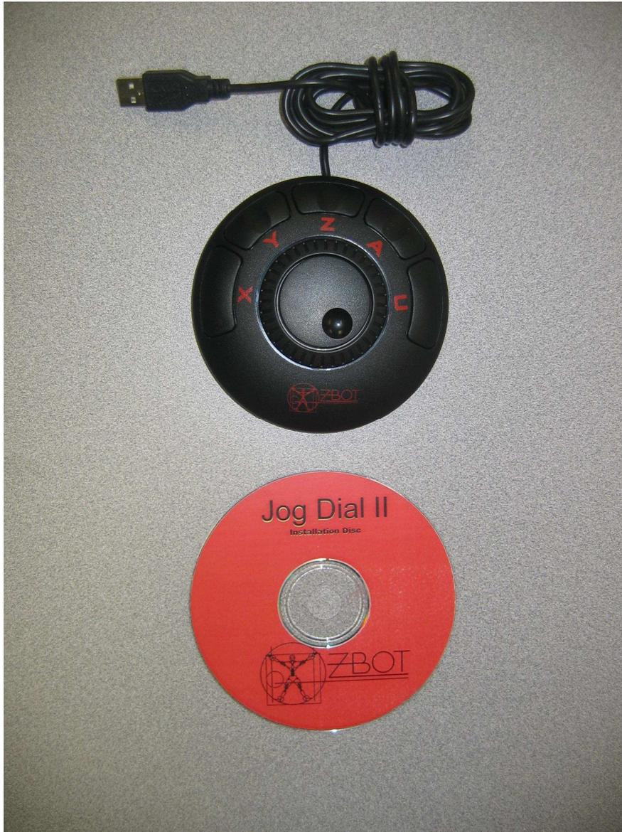
The Z-Bot Jog Dial II is a USB jog pendant controller developed to work in conjunction with the popular Mach3 CNC control software. It is supplied with an installation disc that contains a Mach3 custom plug-in. The Jog Dial II is highly flexible, easy to use, requires minimal configuration, and does not use any parallel port pins.
